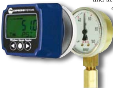
The Wireless Gauge Reader from Cypress Envirosystems digitizes the needle reading and transmits it wirelessly to a central server.
